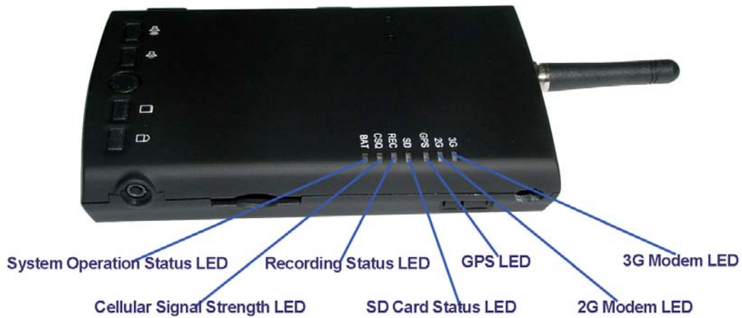
Fig. 3 LEDs on 3G/GPS Camera
